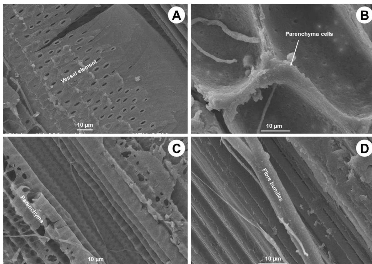
**Figure 2.** A, Vessel element with pits; B, Thick-walled parenchyma cells; C, Thin-walled parenchyma cells with numerous pits; D, Region of fibre bundles.
