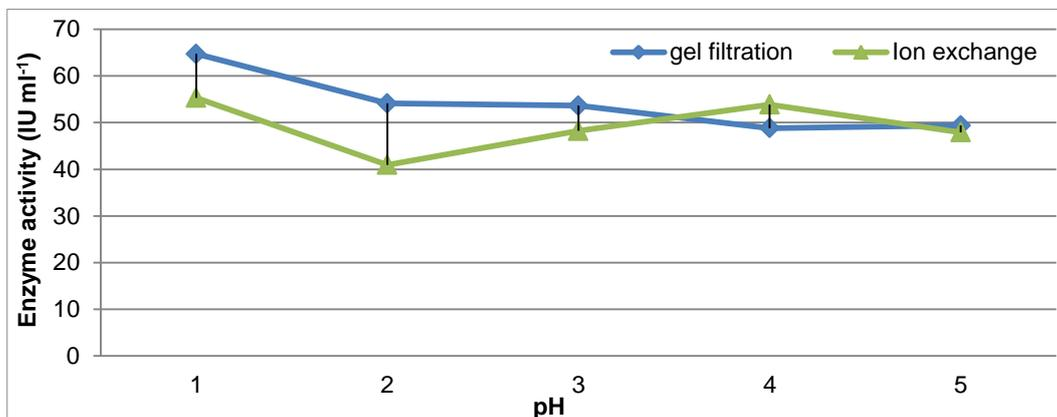
**Figure 3.** Effect of pH of supporting buffer on enzyme purified through gel filtration and ion exchange chromatography (1.0–4.0, 2.0–6.0, 3.0–8.0, 4.0–10.0, 5.0–7.2).
