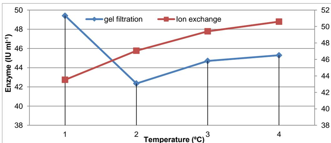
**Figure 4.** Effect of temperature on enzyme purified through gel filtration and ion exchange chromatography (1–30 °C, 2–37 °C, 3–45 °C, 4–50 °C).
